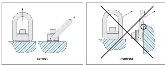
Do not allow the lifting ring to bind/stick and hence apply side loads to the bail. Ensure loads applied are in the same direction of the bail. If necessary use a spreader bar to avoid binding.
