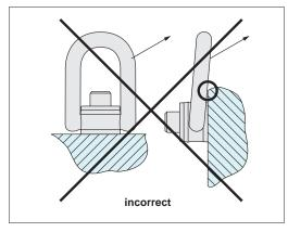
Do not allow the lifting ring to bind/stick and hence apply side loads to the bail. Ensure loads applied are in the same direction of the bail. If necessary use a spreader bar to avoid binding.
