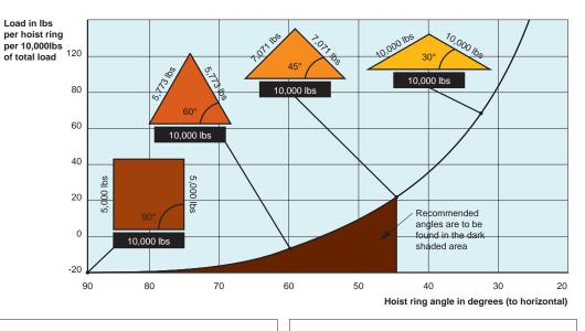
Important note: The force exerted on each hoist ring is not simply a function of the total weight divided by the number of hoist rings, but is critically reliant upon the lifting angle, greater forces are present the lower the lifting angle. See example below.
