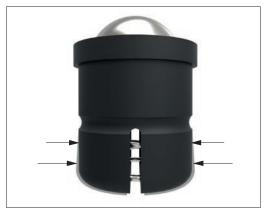
Unique body design flexes to expand and contract to fit in location bore tolerances as wide as +0,2mm. Especially suited to installation in plastic moulded components where hole and bore precision is not high.
