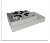
Run first operation – note the clear tooling path possible with no noticeable external clamping interference.
