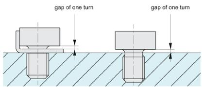
tighten spiral cam clamp fully and loosen it about one turn
