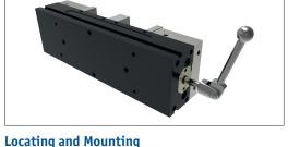
Locating and mounting options are simple and accurate. The bottom surface of the system has four precision dowel pin holes for locating and four drilled and counterbored holes drilled through from the top surface for rugged mounting. Side clamp slots are also incorporated.
