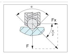
**Important Note: This is only** an approximation formula. For more accurate calculation the roughness of the counterpart surface as well as any variation in the plungers spring force (due to age or high repetitions) should be considered.
