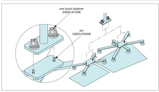
**Changes of Suction Grippers for Wafer** Handling
