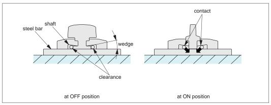
You can slide the steel bar when the knob is at the "OFF" position since there is clearance between the steel bar and the shafts.
