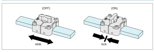
The steel bar can slide to right and left at the "OFF" position.
