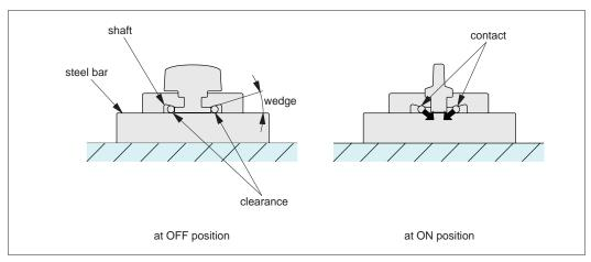
You can slide the steel bar when the knob is at the "OFF" position since there is clearance between the steel bar and the shafts.
