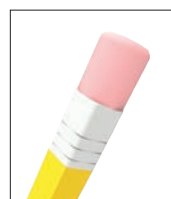
35 durometer: Pencil rubber top
