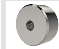
Stainless Steel Pad from 17-4 stainless steel, hardened to Rc 43/46. Mount via tapped or counter bored hole.
