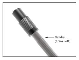
"Pull" Expansion sealing plugs. Pulling on the mandrel expands the sleeve, sealing the channel. At a predetermined force the mandrel breaks off.
