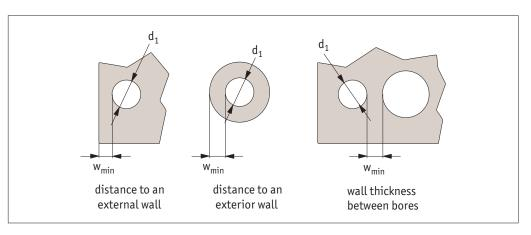
The guidelines for minimum wall thickness or distance from and edge (W<sub>min</sub>) are shown below – these minimum values produce only a very slight deformation on the exterior profile (less than 20 microns).
