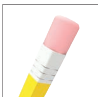
35 durometer: Pencil rubber top
