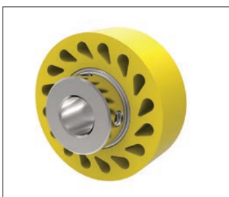
Durossoft rollers - have a smooth contact surface with teardrop holes to allow greater roller compression under load.
