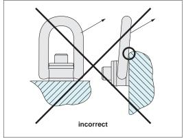
Do not allow the lifting ring to bind/stick and hence apply side loads to the bail. Ensure loads applied are in the same direction of the bail. If necessary use a spreader bar to avoid binding.
