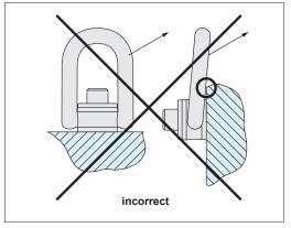
Do not allow the lifting ring to bind/stick and hence apply side loads to the bail. Ensure loads applied are in the same direction of the bail. If necessary use a spreader bar to avoid binding.
