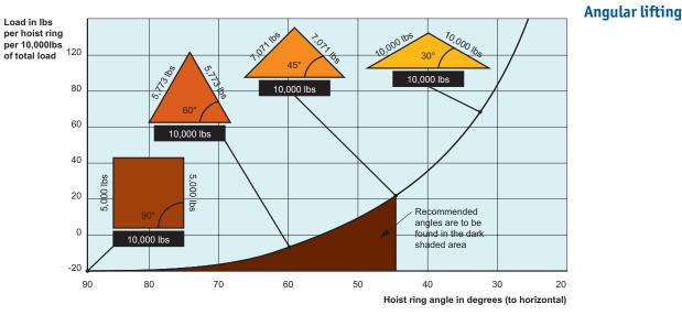
Important note: The force exerted on each hoist ring is not simply a function of the total weight divided by the number of hoist rings, but is critically reliant upon the lifting angle, greater forces are present the lower the lifting angle. See example below.
