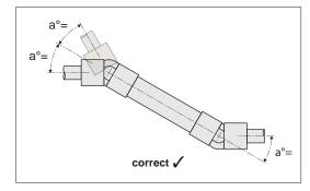
It is essential that the two bending angles a° are equal.
