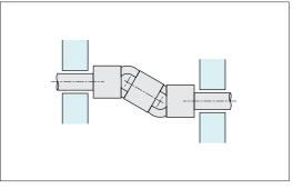
The pillow block supports should be positioned as close as possible to the joints.
