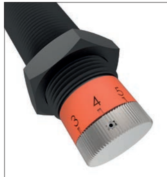
Set collar to 0 at initial installation
