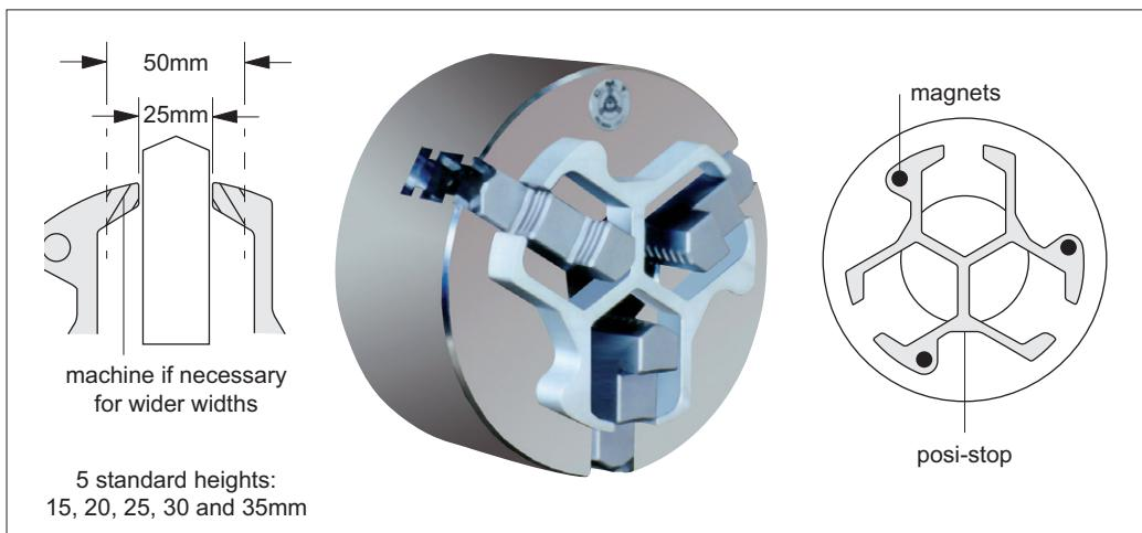
Chuck "Posi-stops" provide a quick and accurate method of moving workpieces away from the face of the chuck. Often used to enable the workpiece to be machined more closely to its extremity or for shorter workpieces.
