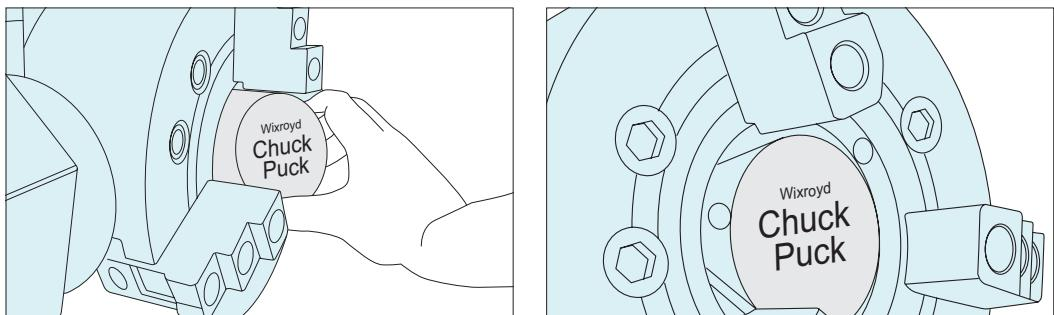
Chuck plug easy to install - just squeeze into the chuck hole.
