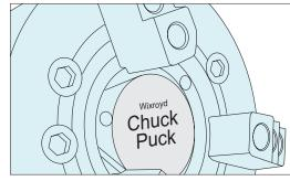
Prevents build up of swarf and coolant, reduces vibration as well as wear of the chuck and spindle.
