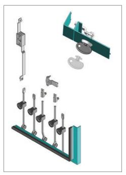
With each multi-point latching system there will be an actuating cam latch, lock or swing handle - attached to these, inside of the cabinet, are a cam and two latching rods.
