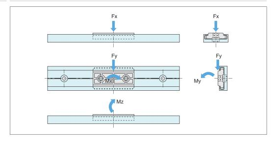
Horizontal static load Fx Verical static load Fy Vertical dynamic load Mx Horizontal dynamic load My Horizontal dynamic load Mx
