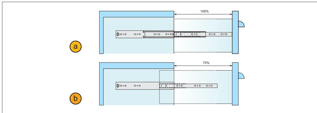
**Full extension** This type of drawer slide can be extended 100% of slide length, this is standard for most 3 piece drawer slides.
