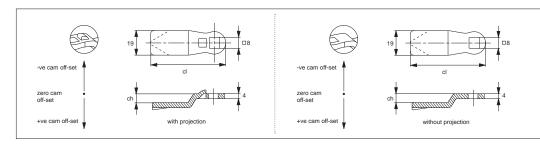
With projection cams prevent turning of the cam over 45°, but is not suited to all cam bodies. For correct projection type please see individual cam body technical pages.
