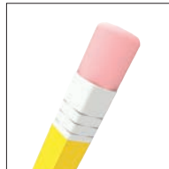
35 durometer: Pencil rubber top
