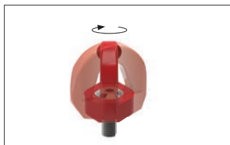
Single swivel - threads M8 – M48 loads 0,3 tons – 15 tons
