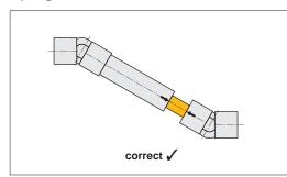
When using two opposite single joints ensure the alignment of the inside yokes.
