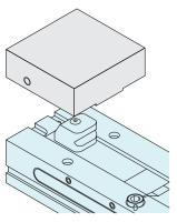
Align the SnapLock outer jaw over the appropriate ReLock vice knuckle
