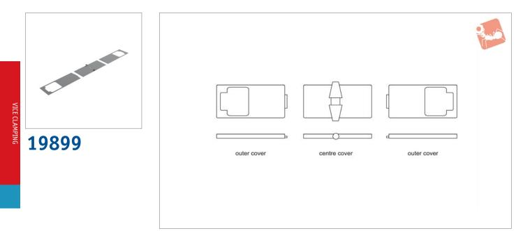
Fits double station and eight station vices. Shield covers protects vice screw and mechanism from swarf and other debris.
