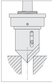
Adjusting the output of the blade controls the thickness of the chip count NOT the value or angle of the chamfer e.g. with a blade protrusion of 0,1mm the chamfering tool requires 10 revolutions to cut 1mm of the chamfer.
