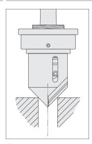
When the chamfer tools spindle is lowered, it's pilot cone firstly centres the workpiece before retracting to allow the blade to come into contact with the material and start cutting of the chamfer.
