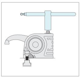
Fix to T-slots with suitable T-nuts.
