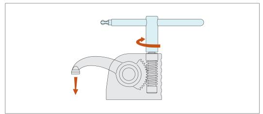
Slide the T-nut into the T-slot position and tighten the clamp onto the T-slot base, with the aid of the clamp key (shown in the image in blue.
