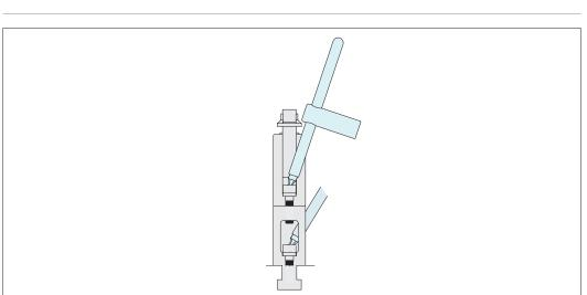
The clamps are easily stackable to achieve required clamping height.
