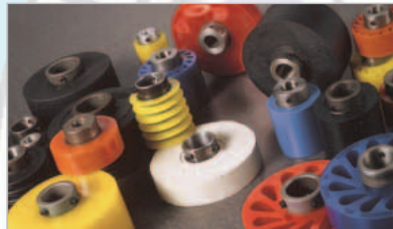
Shaft drive rollers are assembled with the hub already in place. Hub extends from one side with two set screws to lock into shaft. Accomodated shaft sizes from 3/8" to 1-1/4".
